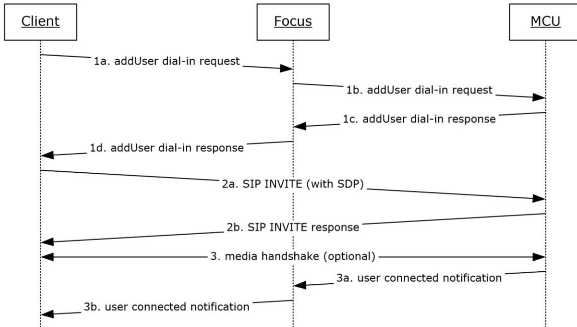
**Figure 16: Connecting a Participant to an MCU**
