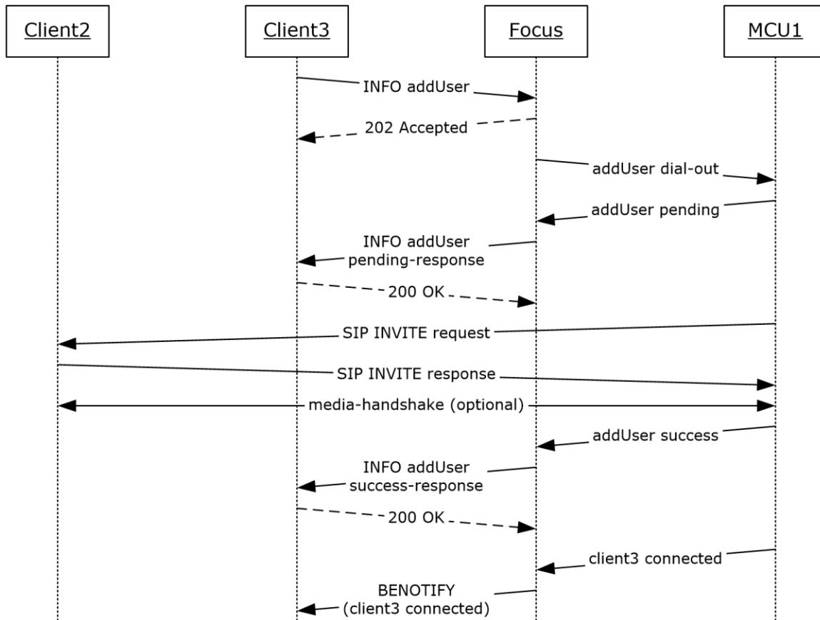
**Figure 15: Connecting a Participant to an MCU**
